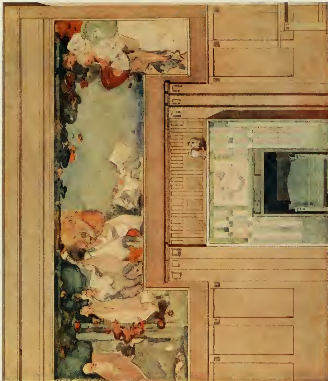
SKETCH FOR A PORTION OF THE DINING-ROOM, PALAZZO REZZONICO, VENICE. MATERIALS: GREY OAK INLAID WITH EBONY, PAINTED PANELS, THE FIREPLACE OF MARBLE AND STEEL.
